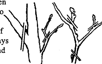
THINNING CUTS Cut to a branch, twig or bud
